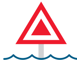
Starboard-Hand Day Beacon: Open red triangle with inner red triangle
