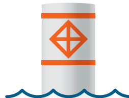
Keep Out Buoy: Orange Diamond with cross on white buoy
