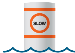
Control Buoy: Orange Circle on white buoy. Mark speed limits, no wake zones
